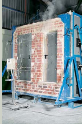
Details of two fire-doorsets in the oven during a fire-resistance test.
