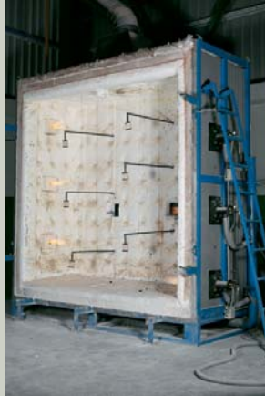
The oven where fire-resistance tests are carried out.
