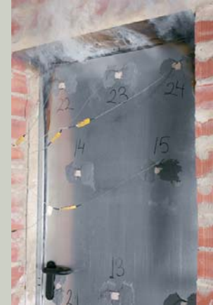
Detail of the thermocouples allowing the control of thermal insulation in fire-doorset during a fire-resistance test.
